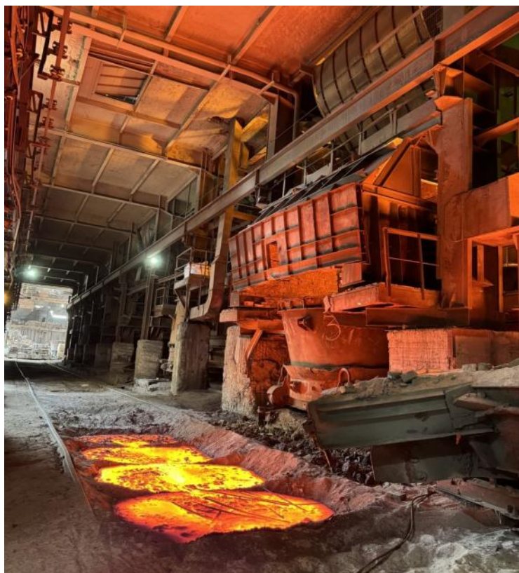
Pictured above are Al 2 O 3 pigs cooling at Zaporizhabrasive.
